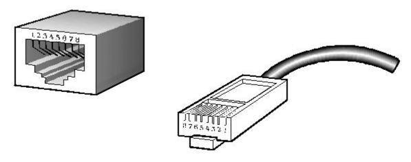
The standard RJ-45 receptacle/connector
